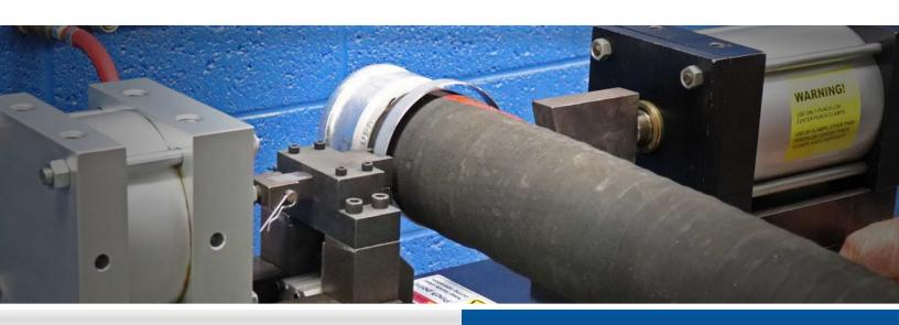
TENSION-AIR™ (TA-3 PLUS™) production hose clamping machines are entirely automatic. Developed by Punch-Lok®, our hose clamping machines eliminate the need for manual punching or bending when applying hose clamps to hose assemblies. Only requiring one person and an average of three seconds to clamp, makes the TA-3 PLUS™ the fastest and most consistent machine on the market for production clamping.
